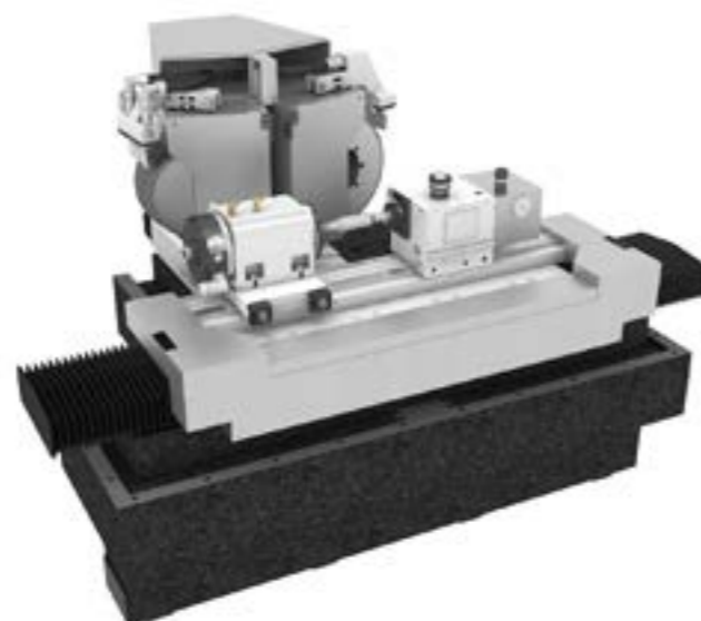
Grinding unit 1: Ø400 x 30 - 0° | Ø15.75 x 1.18 in Grinding unit 2: Ø400 x 120 - 20° | Ø15.75 x 4.72 in
