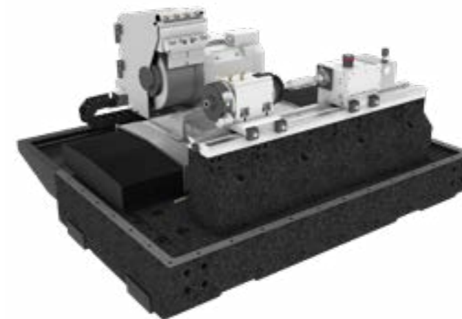
Grinding unit 1: Ø400 x 250 mm | Ø15.75 x 9.84 in
